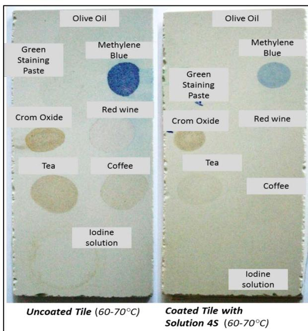
**Figure 2.** Comparison of the stain resistance test between uncoated tile and coated tile with solution 4S at (60-70°C).
