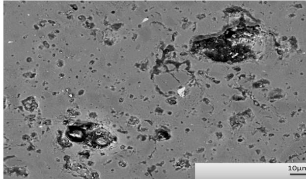
**Figure 7.** The microstructure of tile which was polished 17 cm distance between polishing heads.
