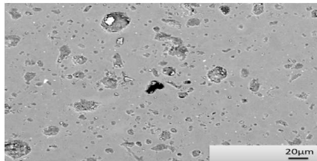
**Figure 4.** SEM micrograph of the tile surface coated with solution 4S at (60-70°C).
