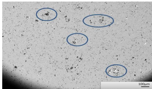
**Figure 9.** The microstructure of polished porcelain tile without soft brushing.
