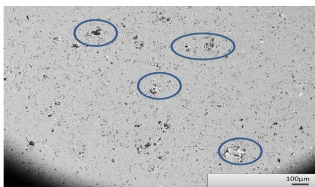
**Figure 9.** The microstructure of polished porcelain tile without soft brushing.
