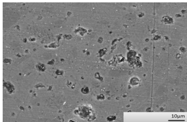
**Figure 8.** The microstructure of tile which was polished 10 cm distance between polishing heads.
