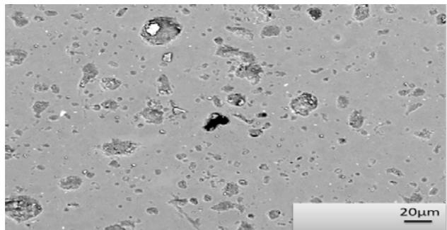
**Figure 4.** SEM micrograph of the tile surface coated with solution 4S at (60-70°C).
