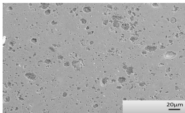
**Figure 5.** SEM micrograph of the tile surface coated with solution 4S at (80-90°C).
