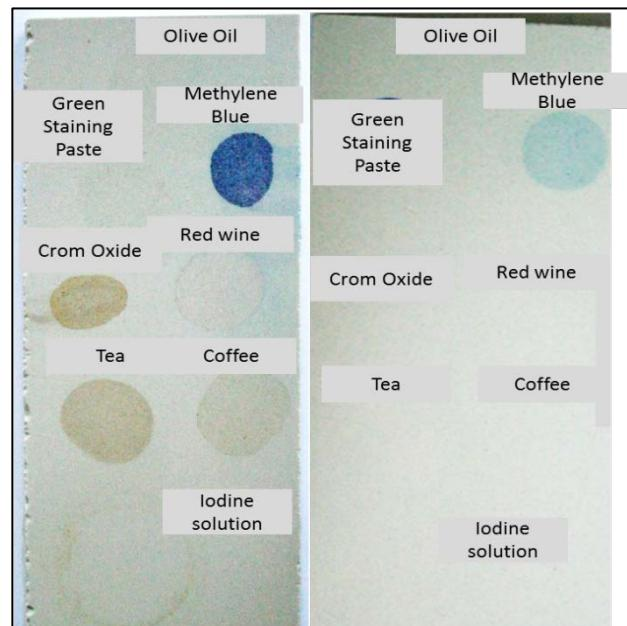
**Figure 3.** Comparison of the stain resistance test between uncoated tile and coated tile with solution 4S at (80-90°C).
