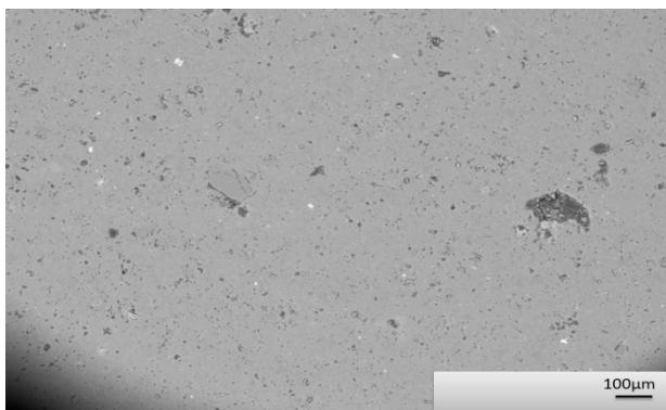
**Figure 10.** The microstructure of polished porcelain tile with soft brushing.
