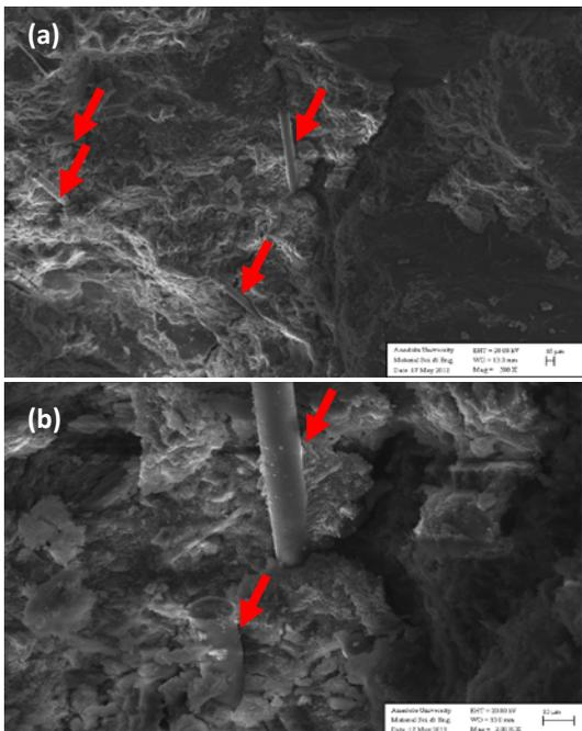
**Figure 4.** (a-b) The SEM images in different magnification taken from the GFRC sample with CA+CFG as 0.5 wt. % at the end of 7 days cure.
