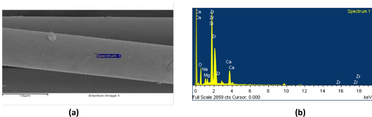
**Figure 1.** (a) The secondary electron (SE) SEM image indicating a place where EDX point analysis on glass fiber was acquired from, (b) The EDX spectrum data coming from marked region in Fig. 1 (a).
