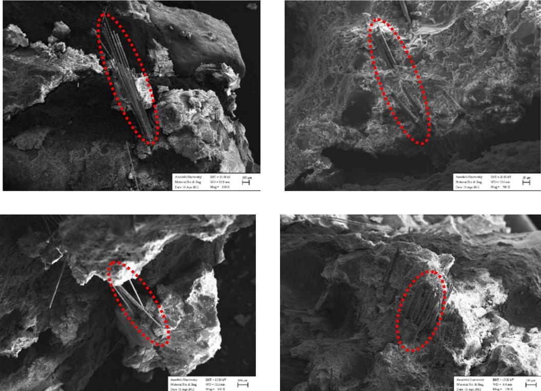
**Figure 3.** (a-b) The SEM images of GFRC samples with the addition of uncoated short commercial glass fibers in 0.5 and 0.7 wt. %, respectively, (c-d) The SEM images of GFRC samples with the addition of uncoated short and long commercial glass fibers in 0.8 wt. %
