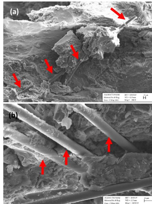
**Figure 5.** (a-b) The SEM images in different values taken from the GFRC sample with CA+CFG as 0.5 wt. % at the end of 28 days cure.
