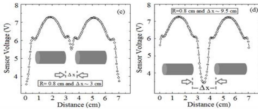
Figure 6. Discontinuities effects on rebar signal
