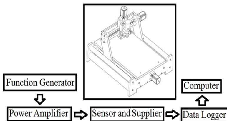
Figure 2. Scheme of magnetic measurement system
