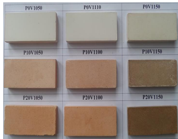
Figure 5. Macro images of non-additive and vermiculite additive porcelain samples.
