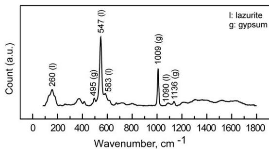
Figure 9. Raman spectrum for the blue sample, B-1
