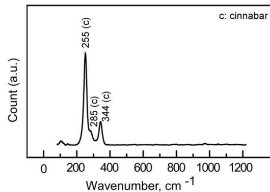
Figure 3. Raman spectrum for the red sample, R-8.
