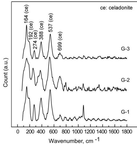
Figure 8. Raman spectra for the green samples
