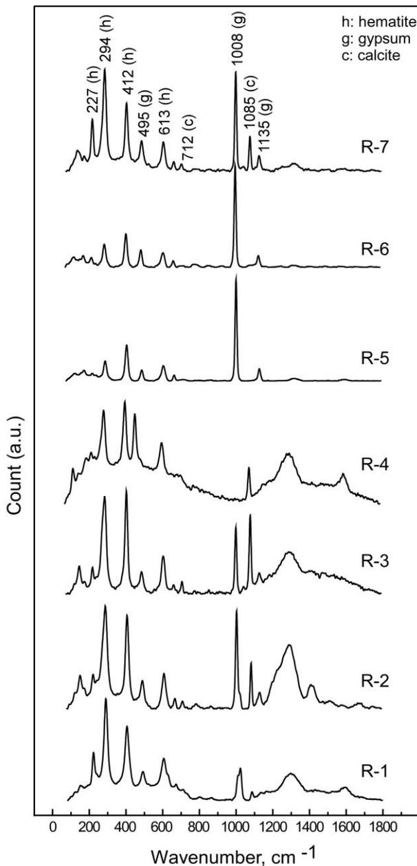
Figure 2. Raman spectra for the red samples (R-1 to R-7)
